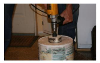
I. Using the hole saw, drill a 4" hole in the bottom of the bucket.
