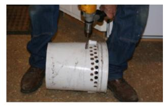
2. Drill a series of holes all over the bucket using the spade bit.
